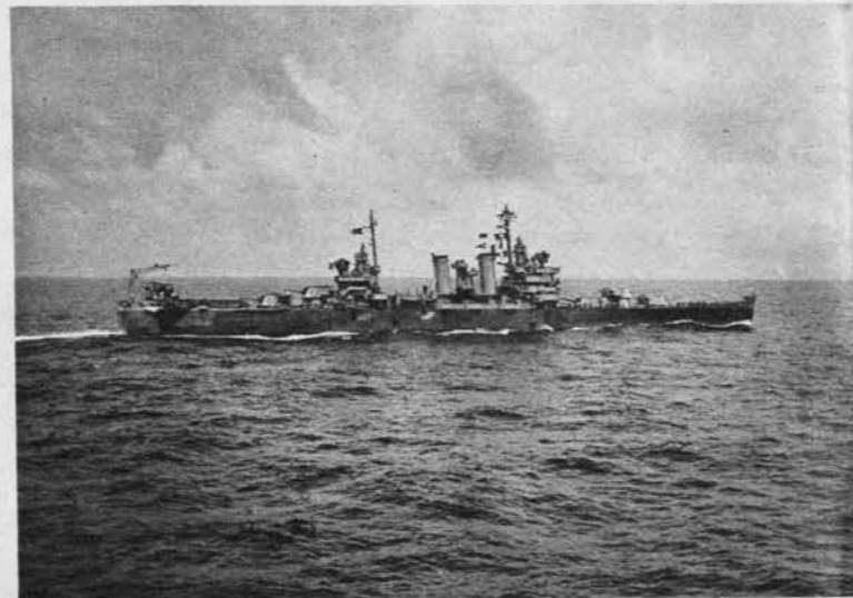
Heavily armed Brooklyns were U. S. answer to Jap Mogamis, have five turrets. Note separated superstructure, stacks set close to bridge.
